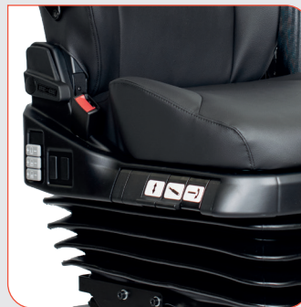
User friendly control panel. Can be left or right side.
