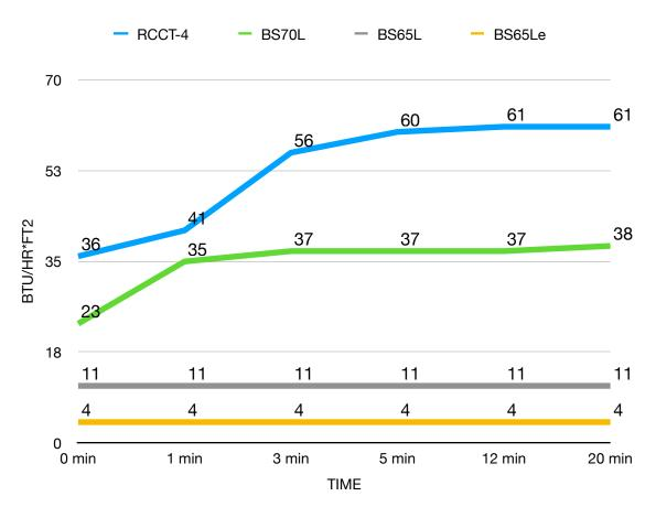
**Test Two:** The meter is positioned 10 inches away from the heat source measuring 300 BTU with no glass barrier. Each glass sample is positioned between the Portable Heat Lamp and Solar Power Meter for 20 minutes while recording the BTU thermo-properties at specific intervals.
